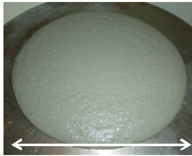
Figure 4 Flow of the mortar mixed by CM-pump
