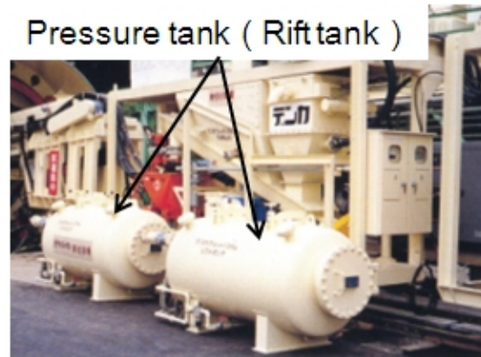
Figure 10 Pressure tank (Rift tank)
